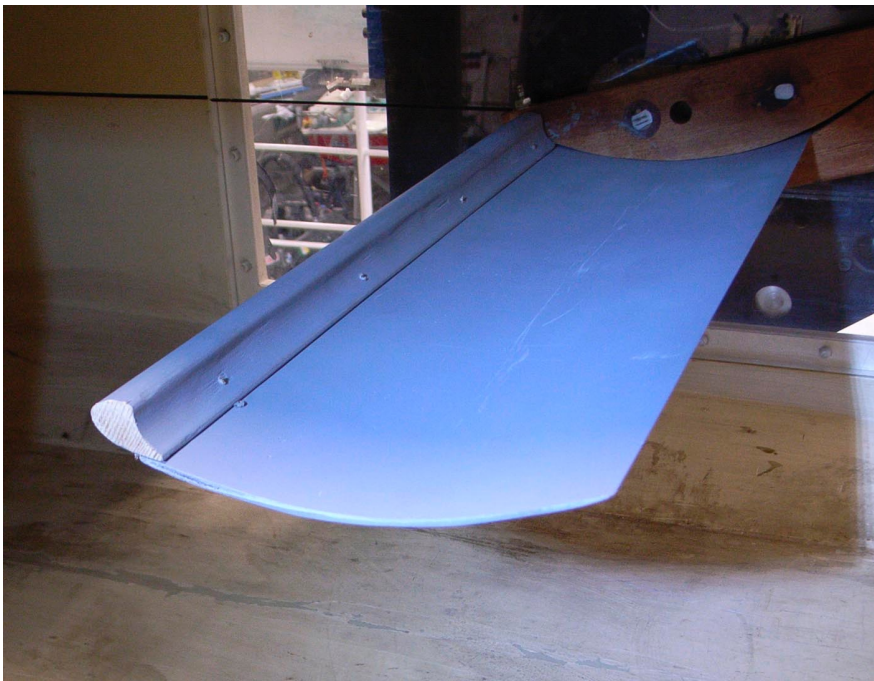
Example of a rigid, 2D wing section model mounted in the wind tunnel. In this case a low camber section fitted with a “WP2” leading edge section.
